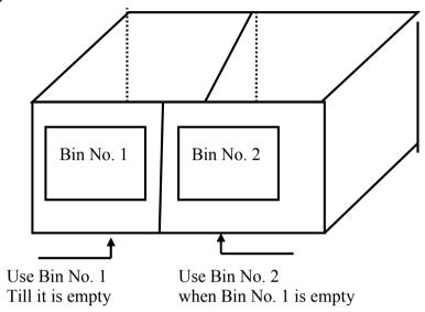
In this system, two bins are used and the stock is divided into two bins. The first one is used for satisfying current demand and the second one is used during the replenishment period. The second bin is used only when the first bin is empty and the replenishment order is placed. When the replenishment order is received, first the second bin is filled and then the balance is put in the first bin.
