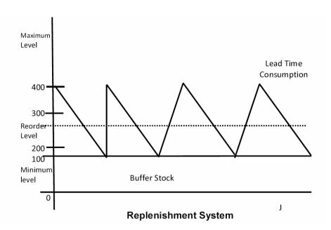
The above diagram represents an average rate of consumption of 100 units per month. The supplies are purchased once in three months (300units). The minimum level/Buffer stock is maintained at 100 units i.e. equivalent to one month's consumption. The lead time, in this case, is 45 days. This means that when the stocks reach a level equal to 45 days consumption above the minimum level, a replenishment order is placed. The re-order level is at 250 units. The maximum stock held is 400 units.
